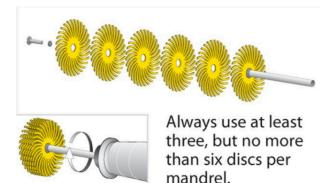
Abrasive discs developed by 3M especially for jewellers. Each flexible plastic disc is colour-coded to indicate the specific grit. No compound is necessary, grit is uniformly dispersed throughout the disc. You work faster and clean-up is much easier!
